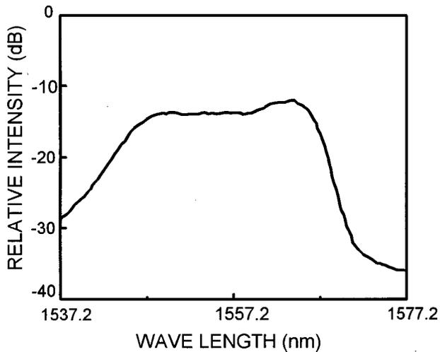
Fig. 5. Time-averaged optical spectrum of the mode-locked laser that corresponds to Fig. 4.
