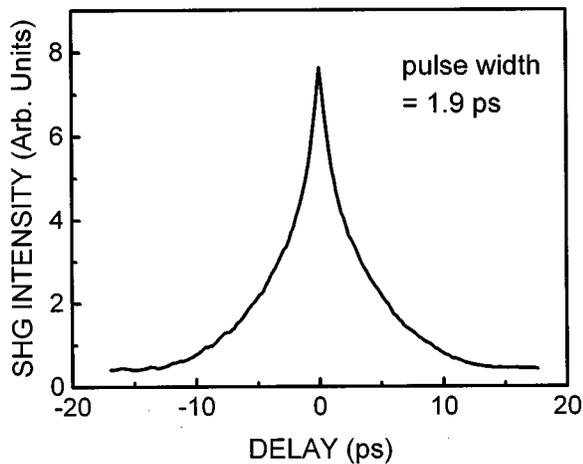
Fig. 4. SHG autocorrelation traces of the output pulses from the mode-locked laser with the SBR in the external cavity.
