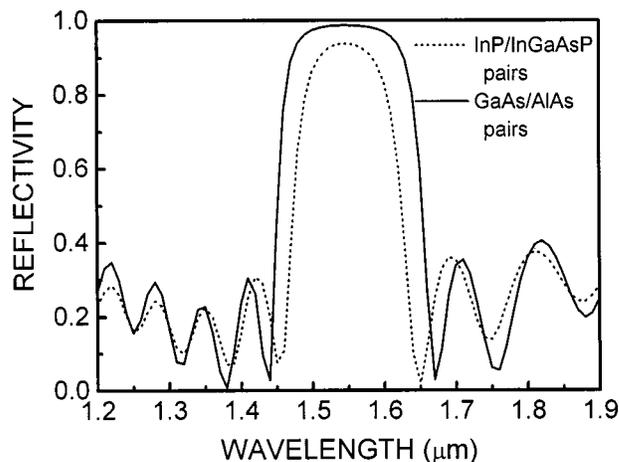
Fig. 2. Reflection spectra of the InP/InGaAsP and GaAs/AlAs Bragg reflectors.
