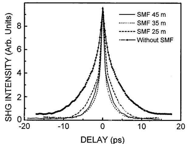
Fig. 6. SHG autocorrelation traces after compression with the SMF at different fiber lengths. The shortest pulse width was found when the SMF length was 35 m.
