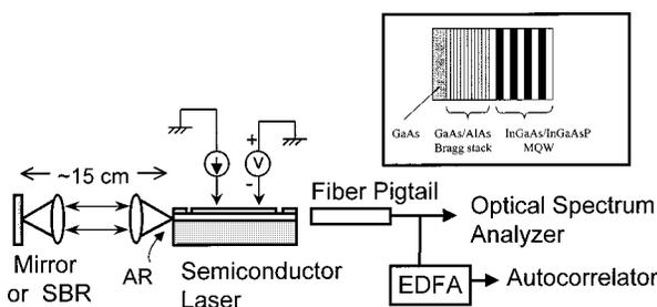
Fig. 1. Schematic of the experimental setup for mode locking with a SBR. Inset, structure of the SBR.
