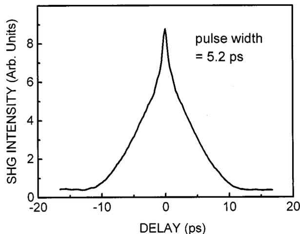
Fig. 3. SHG autocorrelation traces of the output pulses from the mode-locked laser with a planar mirror in the external cavity.
